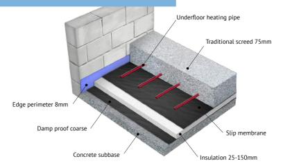
Compared with other liquid screeds which generally need to be force dried with underfloor heating; Cemfloor screeds can be used in non heated floors as it doesn't require force drying to remove moisture. Using the correct tile adhesives; tiles can be placed in as little as 5 days in nonheated floors.
